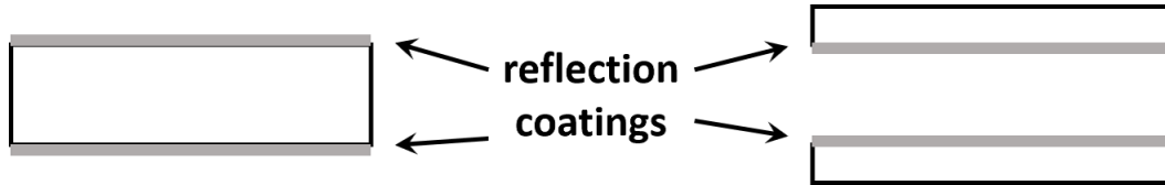
Fig. 2.13: Types of Etalon constructions.
